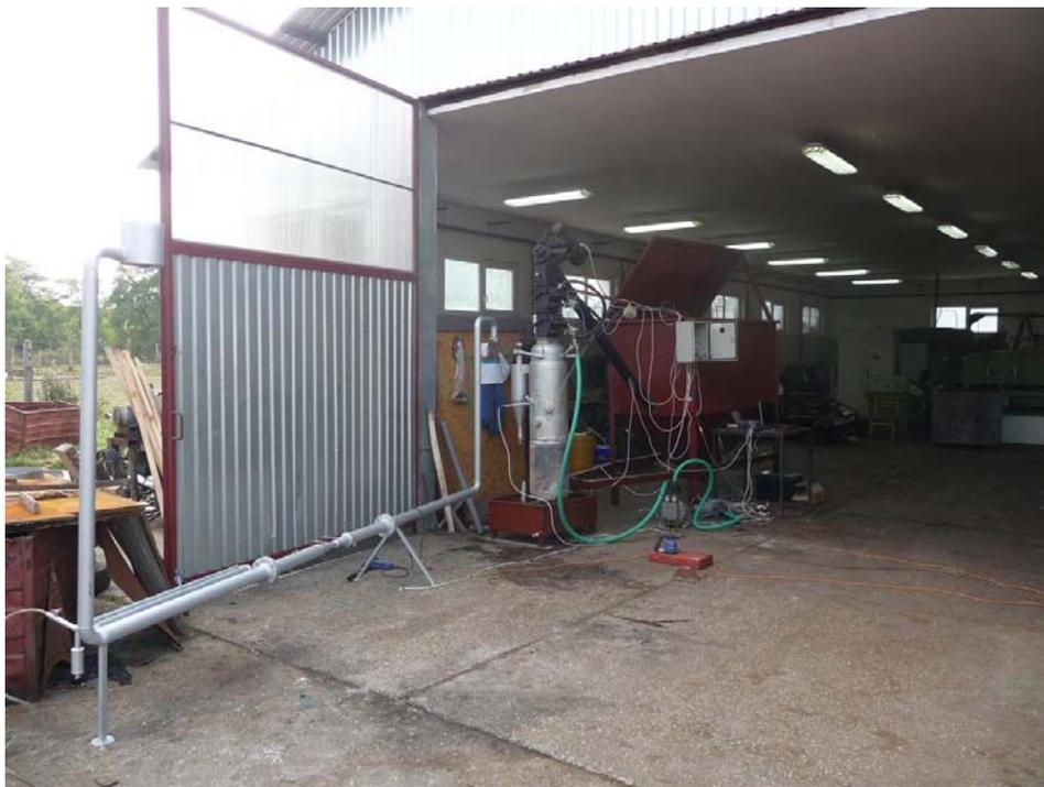
Fig. 3.: The gasifier prepared for measurements with the woodchips container and the measurement system.
